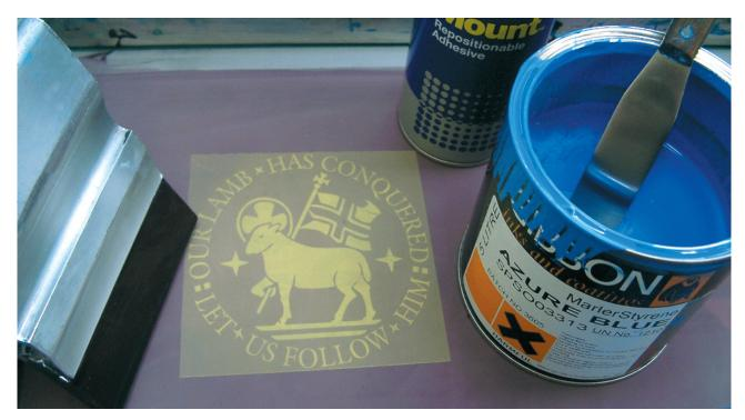
Screen printing is available on most sheet metals, plastics and vinyls. We stock various ink systems in all the standard colours. Any colour can be matched to a BS or RAL number, or to a customers sample. This economical and versatile process can be used to print an array of 'free issue' products providing the surface to be printed is flat, clean and dry.
